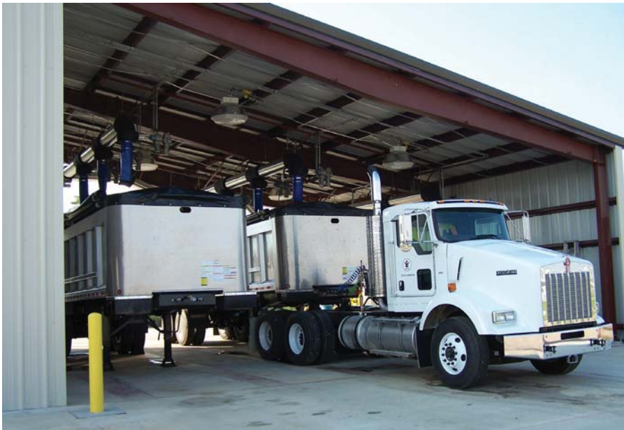
Above: Fisher & Arnold's engineers developed a design space that provided for three trucks or containers to receive the dewatered sludge.
